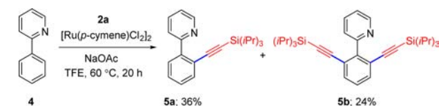
Scheme 2. Ru-Catalyzed C–H Alkynylation of 2-Phenylpyridine
